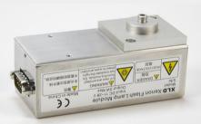
High power is beneficial to improve the signal-to-noise ratio Wide spectral range of 185-2000nm, covering UV, VIS, NIR Long life, more than 100 million flashes Good stability, CV value of 1000 flashes ≤ 2% Small size, low heat No-preheat, work immediately Plug and play DB-9 connector
